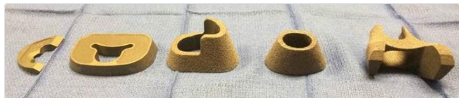
(Top): Examples of metal augments that can be added to implants to make up for lost bone.
